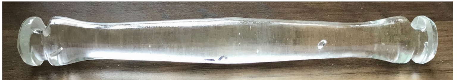
STYLE 3: UNEMBOSSED, THICKER "NECK" WITH ASYMMETRICAL WIRE GROOVES (SQUARE AND ROUND). PHOTO COURTESY CONNIE DUEKER.
