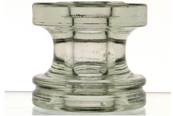
ABOVE: UNLISTED CD 1052 HEMINGRAY-518 EMBOSSED WITH A SMALL MOLD NUMBER "5". THIS PIECE ALSO HAS AN UNTHREADED BOLT HOLE (VERY UNCOMMON FOR A HEMINGRAY EMBOSSED PIECE). PICTURED UPSIDE-DOWN TO SHOW THE MOLD NUMBER.
