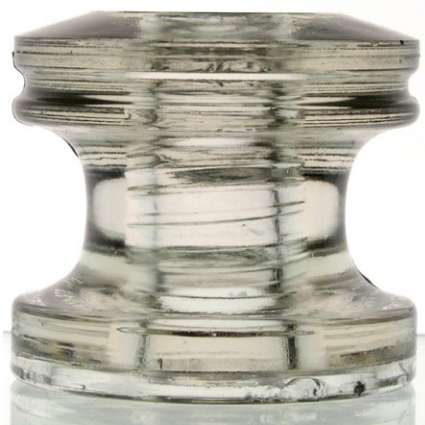
ABOVE: HEMINGRAY-518 "TAPER TOP" MOLD VARIANT. NOTE THE SLOPED TOP. THIS PIECE ALSO HAS THE UNCOMMON, LARGER 3/16" EMBOSHING STYLE (SEE MIDDLE PHOTO ON RIGHT)
