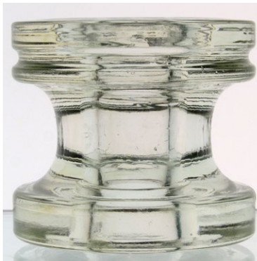
NO EMBOSHING [010] CLEAR UNTHREADED BOLT HOLE
