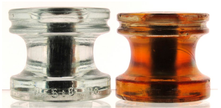
ABOVE, LEFT: TYPICAL NO NAME D_518 IN ICE BLUE WITH LEAD BUSHING. ABOVE, RIGHT: NO EMBOSHING "MINI MOLD" VARIANT, WHICH IS ABOUT 1/8" SMALLER IN HEIGHT AND WIDTH; ALL SPECIMENS I'VE SEEN SO FAR ARE CARNIVAL, HAVE AN UNPUNCHED BOLT HOLE, AND A METAL SLEEVE INSTALLED. THESE WERE CLEARLY DUMP PIECES; POSSIBLY A PROTOTYPE OF THE FINAL CD 1052 DESIGN?
