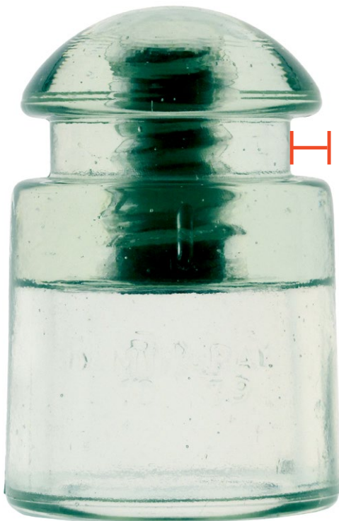
FRONT VIEW OF [080]: WIRE GROOVE APPEARS SHALLOW; VERTICAL BARS ON FRONT & REAR
